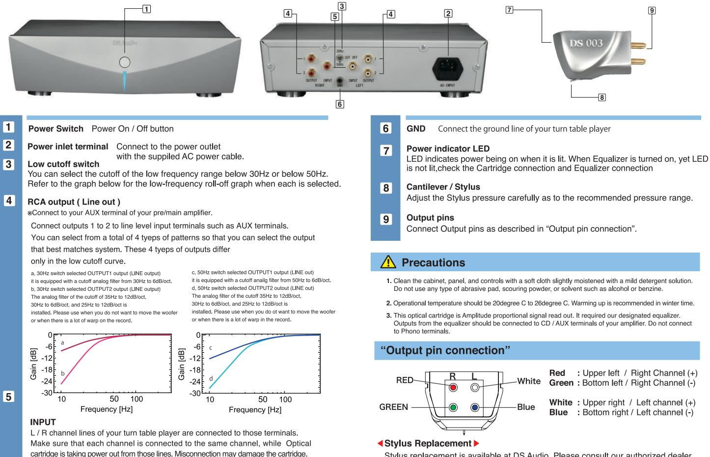
\*Do not connect MM/MC cartridge to this Equalizer. It may break MM/MC cartridge.
