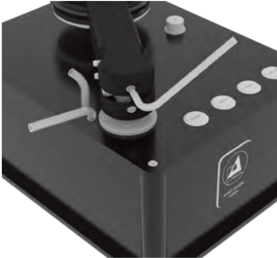
Pic. 13: Disconnecting the hoses
