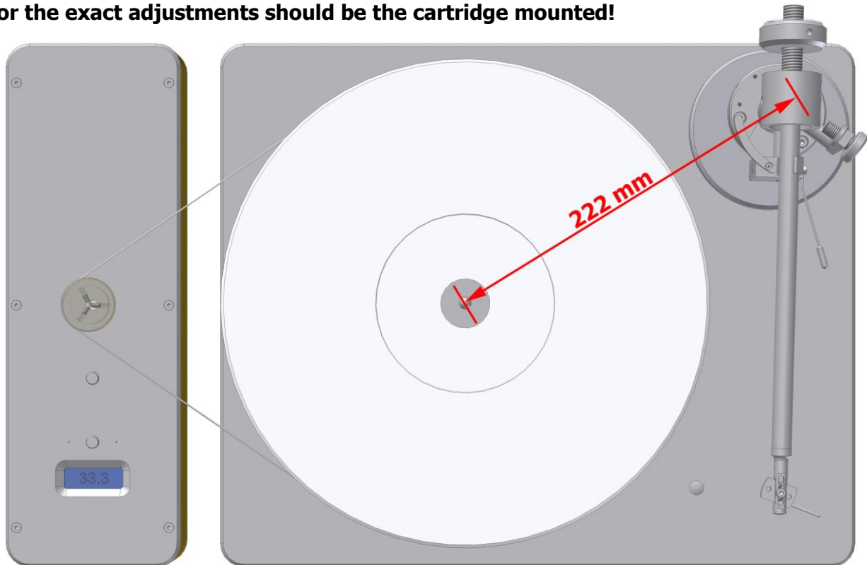
Picture 3: Distance from pivot to stylus
