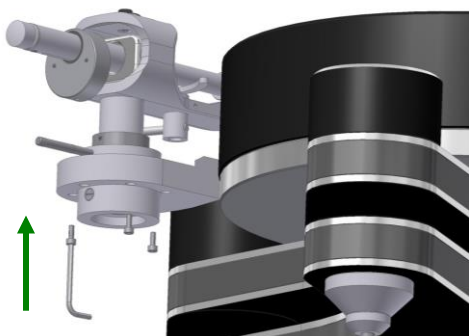
Pic. 3: Set-up of tonearm base with VTA-Lifter
