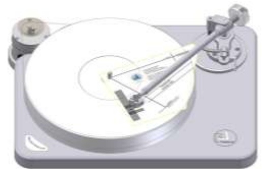
Pic 8: Alignment of the tonearm
