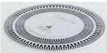
To adjust the exact speed, please choose the side for 50 / 60 Hz, or the other side for the use with the speed light first. If you choose the side without the speed light source, you can use the regular light source for the installation, either 50 Hz (outer scales) or 60 Hz. The scales are graduated in three different reading options: 33.3 Hz, 45 Hz and 78 Hz (starting from the outer diameter).
