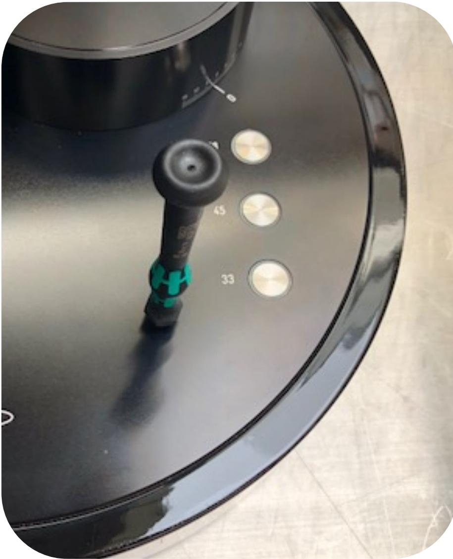
After the platter and tonearm are installed, re-position the turntable to the point where it will be used. Final leveling can be done using the 3mm hex driver and the 2 spike feet which remain accessible. Use the built in bubble level to ensure the turntable is properly level. At this point you are ready to proceed with the installation of the tonearm's counterweight and cartridge, following instructions provided in the tonearm manual and by your cartridge manufacturer.
