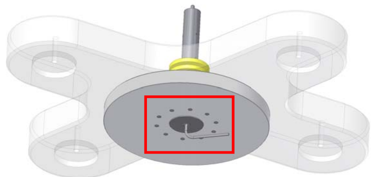
Pic. 15: To attach the upper drive platter to the bottom of the main bearing spindle
