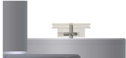
Pic. 20: Setting the motor pulley
