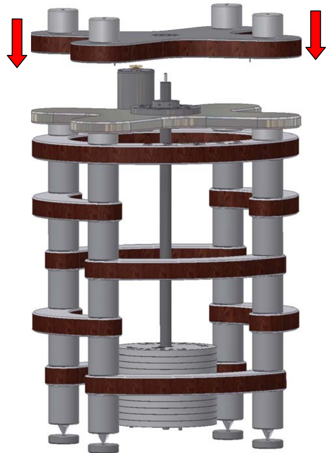
Pic. 9: Removing the wooden spacers
